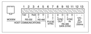
Figure C-6 The Communications Terminal Block
